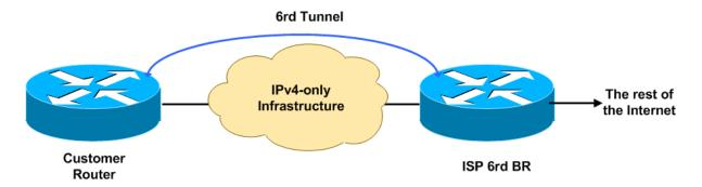
The Customer Router in the diagram is our Customer Router in our network. And the ISP 6rd BR capability will be configured on our autonomous system's Border Router.
