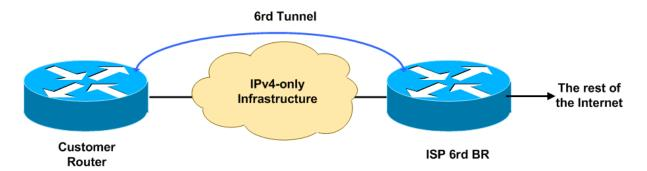
The Customer Router in the diagram is our Customer Router in our network. And the ISP 6rd BR capability will be configured on our autonomous system's Border Router.
