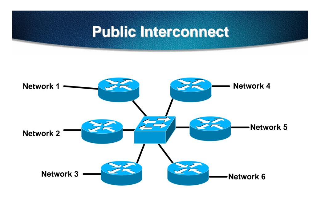
each of these represents a border router in a different autonomous system
